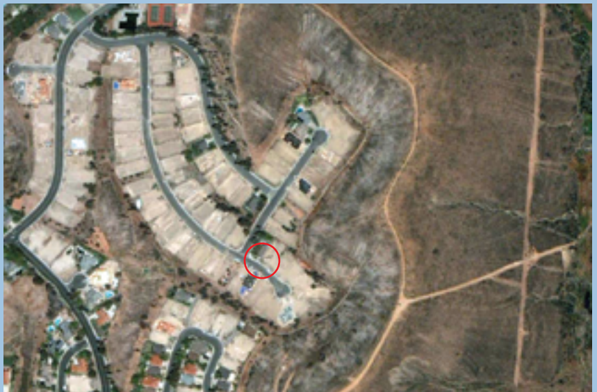
Few homes survived the 2003 Cedar Fire as it ravaged the San Diego, California, community of Scripps Ranch, shown here after the fire. One of the remaining homes (circled) had just had its wooden roof replaced with a fire-resistant one, against the wishes of the local homeowner’s association. Studies have shown that structures with wooden roofs can be up to 20 times more likely to be destroyed in a wildfire, depending on their distance from flammable vegetation. (Image courtesy of Richard Halsey.)
